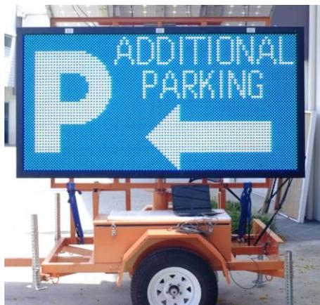
include a solar power option and incorporate reliable communication interfaces meaning that the sign can be placed almost anywhere and remotely programmed.
